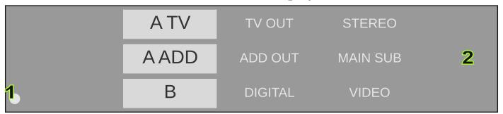
1 The small circular indicator illuminates when a valid remote control command is received.
